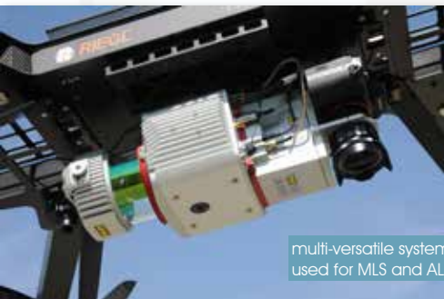
RIEGL VUX-1UAV LiDAR Sensor equipped with APX-20 UAV, Flir Tau 2 thermal camera, and Sony Alpha 7R III camera
