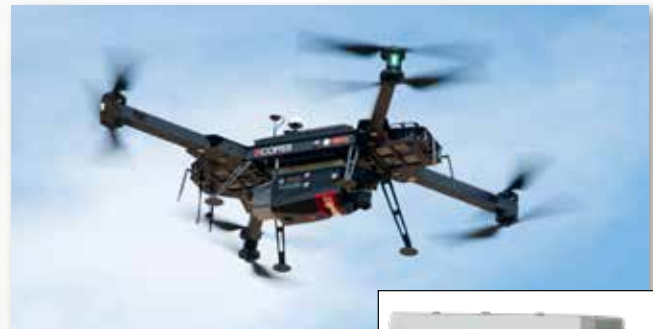
RICOPTER with RIEGL VUX-240 LiDAR Sensor, APX-20 UAV and nadir RGB camera fully integrated
