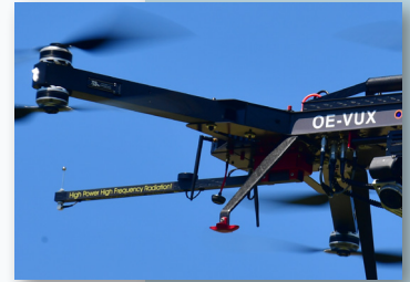
RICOPTER-M equipped with ADS-B/Mode-S transponder
